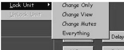
B.Lock Unit provides four options for security lockouts in the pull-down menu. Make your selection and enter your password in the text box. You will then need to confirm the password and OK the lockout. To unlock the unit, under the Device menu, click on Unlock Unit. Enter the password in the text box and click OK. Then click on the Clear Password box.
