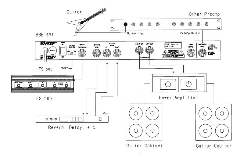
The BBE 651 Guitar Pre-amp may be configured with one or more guitar pre-amps to achieve new and exciting tones. Experimentation is suggested to determine which pre-amp shall be first in the signal chain. Note: The  $SVC^{tm}$  circuit should be in the "OFF" position when the BBE 651 is being used with guitar speaker cabinets.
