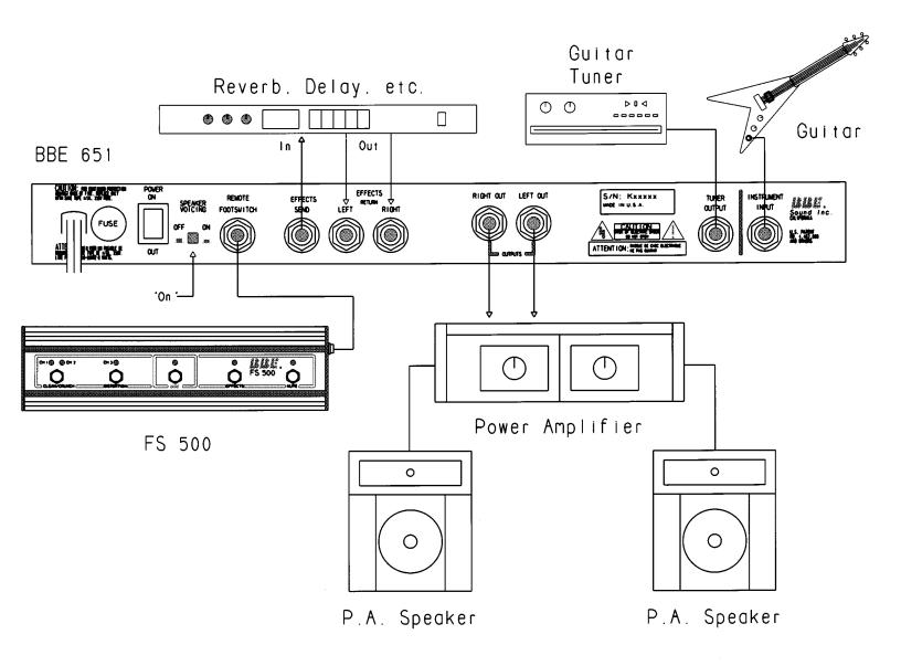
The BBE 651 Guitar Pre-amp may be connected directly into a mixer or into a power amp (as illustrated) and still maintain a warm guitar cabinet sound with the use of the  $SVC^{tm}$  circuit.
