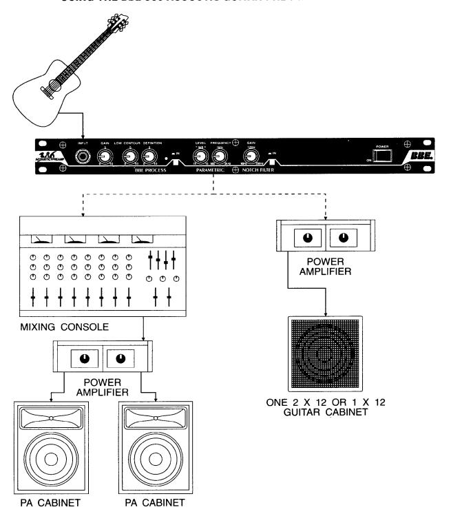
In the past, to be heard properly, an acoustic guitar had to share the same amplifier as an electric guitar. It worked, but did not compliment the acoustic guitar too well. Now, with the addition of the **BBE 386 Acoustic Guitar Pre-amp**, proper amplification of the acoustic guitar can be achieved.
