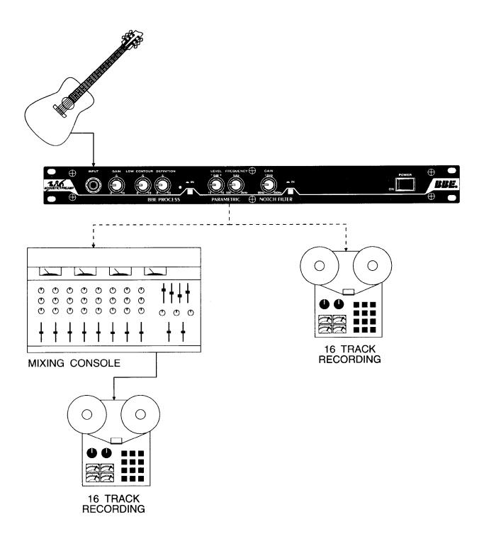
The **BBE 386** is a great way to amplify an acoustic guitar signal to an adequate recording level. With its low noise level, the **BBE 386** can be connected directly to a tape recorder for the purest sound possible or through a mixing console for the addition of effects or secondary tone modification.
