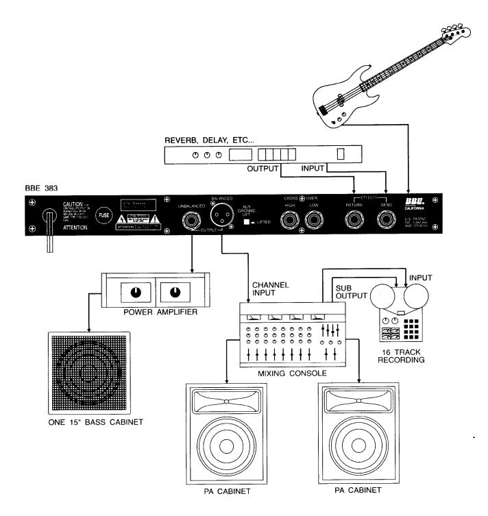
For most configurations, using the **Unbalanced** output of the BBE 383 Bass Guitar Pre-amp to connect to a speaker cabinet for monitoring the bass guitar and using the **Balanced** output to connect to a mixing console for live and studio applications will prove to be an ideal starting point.
