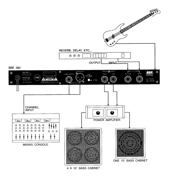
Use the **Crossover** outputs for configuring a more sophisticated system. An advantage to **Bi-amping** is that each speaker cabinet is working on a smaller frequency band than a full range output. The speakers then work more efficiently and produce better results. The main outputs and the **Crossover** outputs are interchangeable and are worth experimenting with to find the ultimate configuration!
